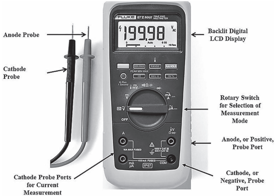
FIGURE 1.27 Fluke® 87 V Max (printed herein and reproduced with permission of Fluke Corporation) True RMS Digital Multi-meter.
